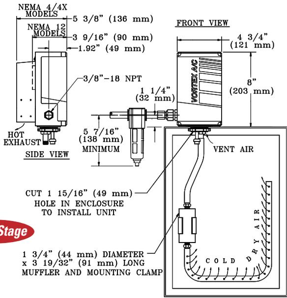
(VORTEX A/C SHOWN TOP MOUNTED ON CUSTOMER'S ENCLOSURE) 900, 1500 AND 2500 BTUH MODELS SHOWN HERE
