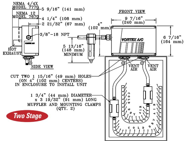
(TWO-STAGE 5000 BTUH VORTEX A/C SHOWN TOP MOUNTED ON CUSTOMER'S ENCLOSURE)
