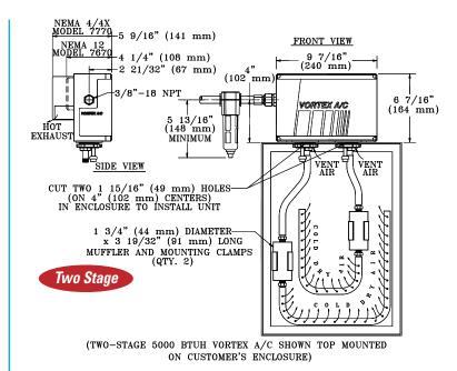
Recommended operating pressure for all Vortex A/C models is 90 to 100 psig (6.2 to 6.9 bar).
